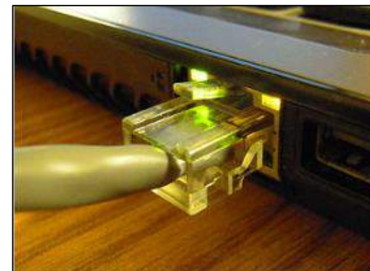
A twisted pair cable with an 8P8C modular connector attached to a laptop computer, used for Ethernet
