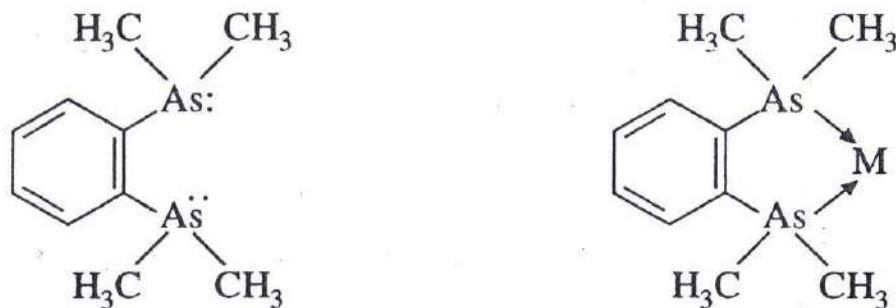
Fig. 1.3. (a) Structure of o -phenylene bis dimethyl arsine (diars or D) (b) Mode of attachment of diars with a metal atom, M in complex compounds.
