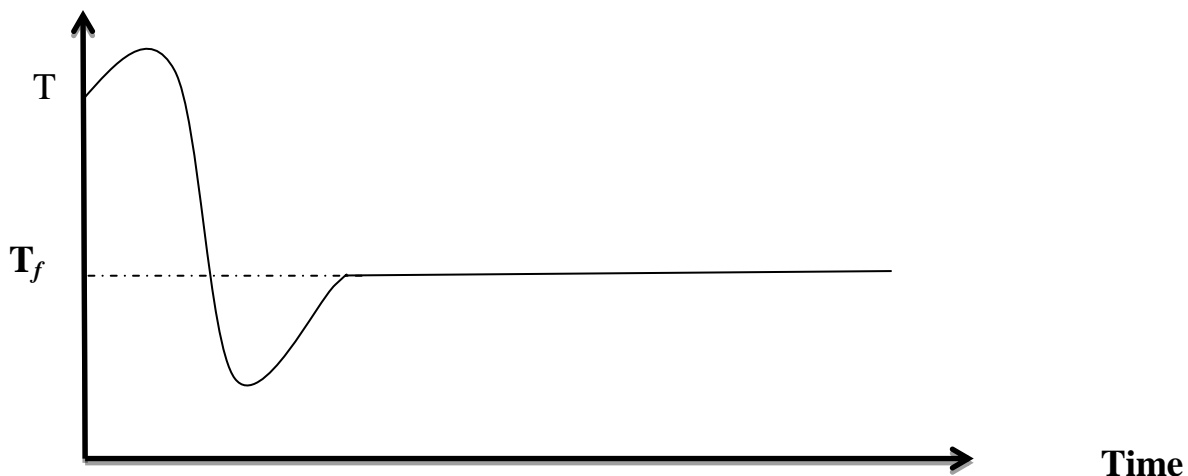
Fig. 4: The halt in the cooling curve results from the heat evolved when the liquid solidified.
