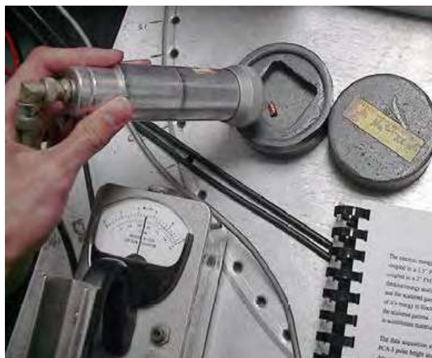
Figure shows: These dosimeters (literally, dose meters) are personal radiation monitors that detect the amount of radiation by the discharge of a rechargeable internal capacitor. The
